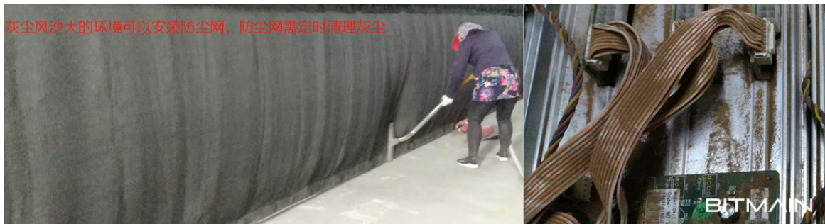
吸尘器清理防尘网、矿机附着沙尘
