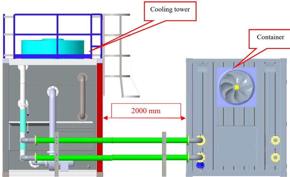
Figure 2-1 The relative position of the container and the cooling tower
