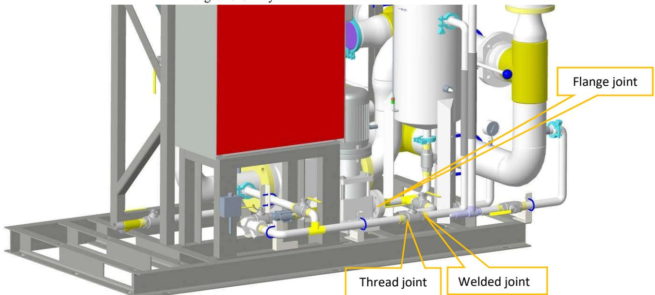
Figure 5-7 System - Flange/thread/welded joints
