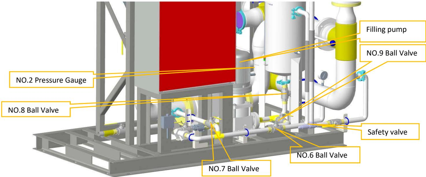
Figure 7-5 Pump station - charging valve
