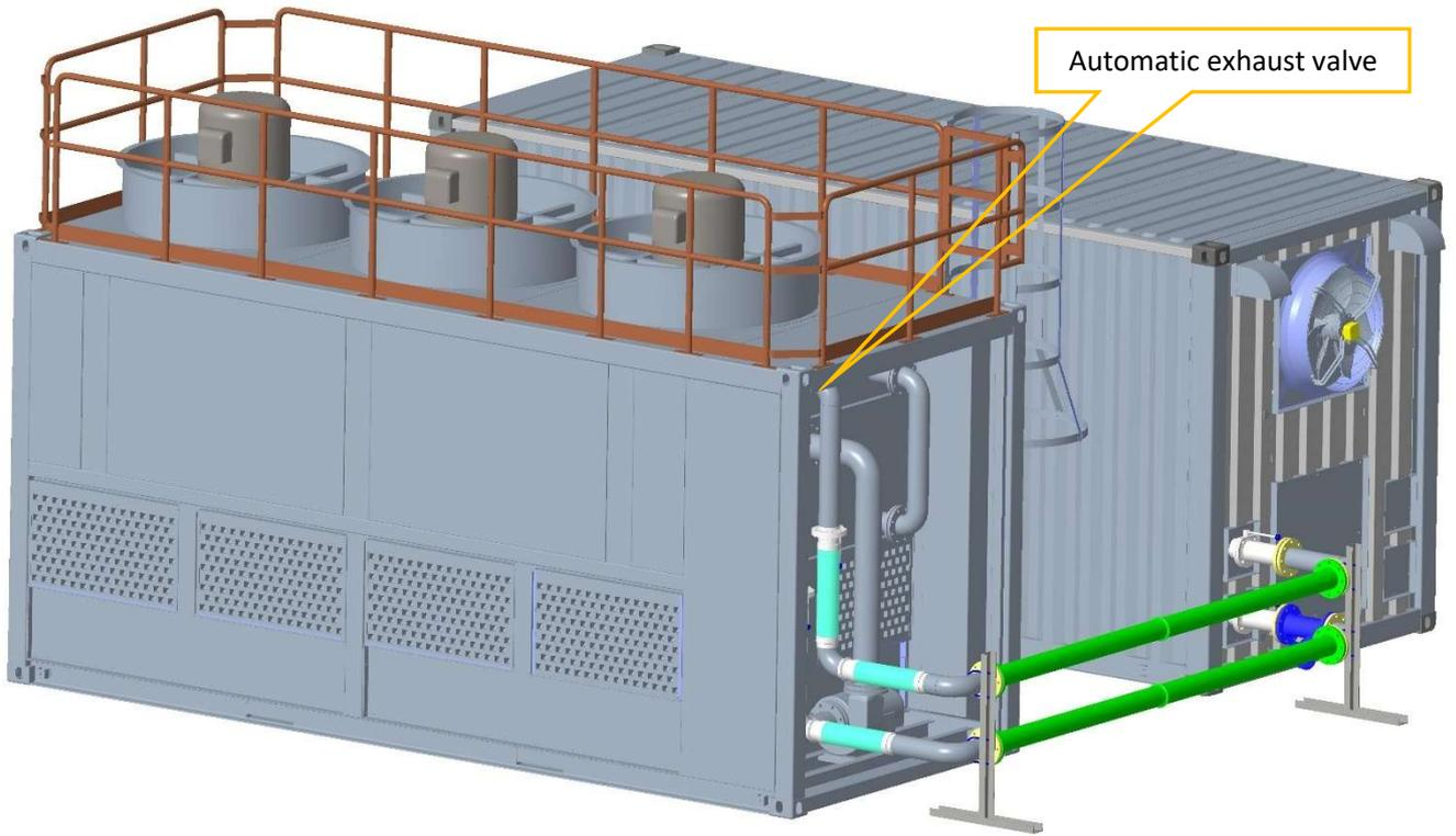
Figure 7-3 External connecting pipelines - automatic exhaust valve
