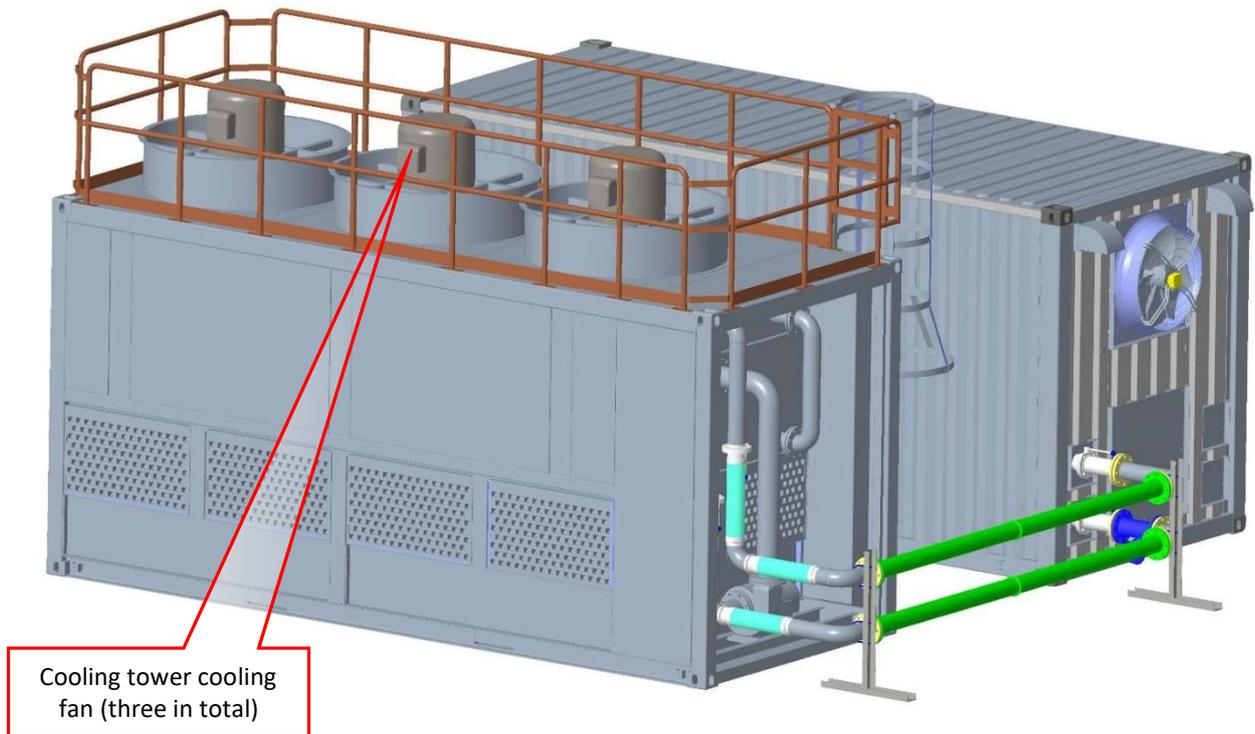
Figure 5-3 Location of cooling tower cooling fan
