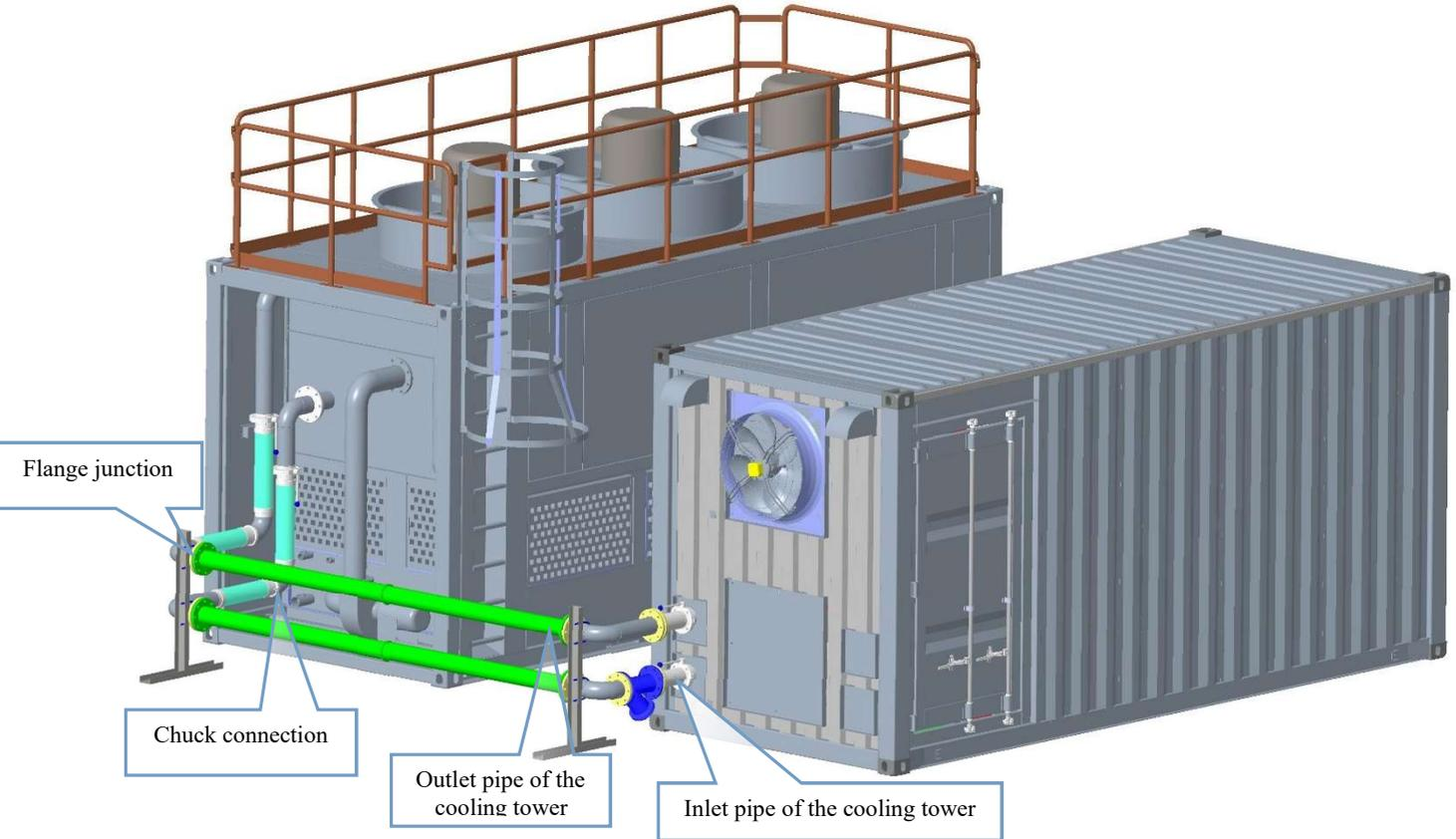
Figure 4-1 Installation of the intermediate connecting pipelines
