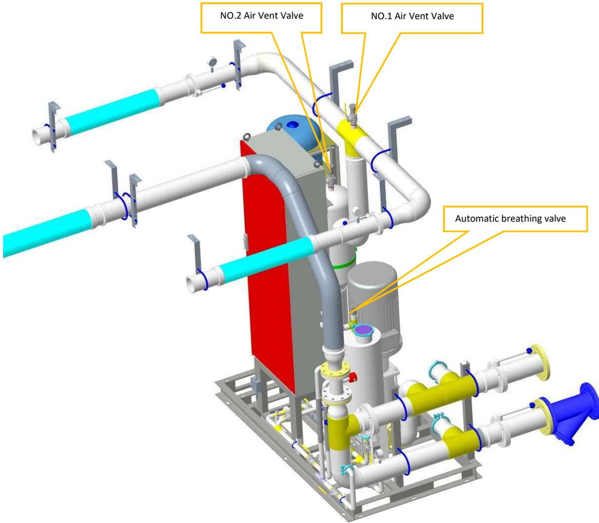
Figure 5-1 Pump station - automatic exhaust valve
