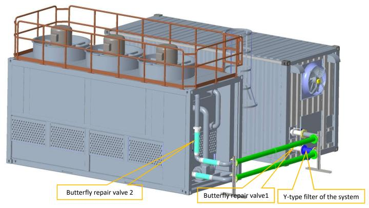
Figure 8-3-1 Positions of the butterfly repair valve and the Y-type filter in the pipelines
