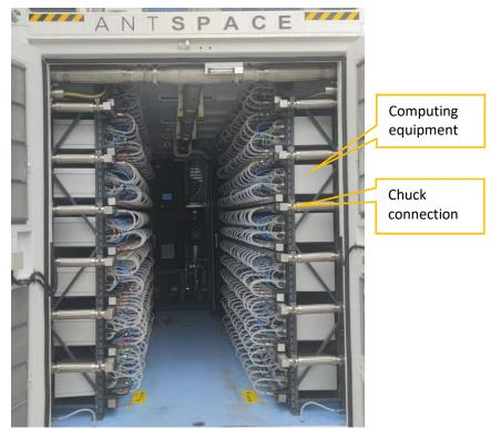
Figure 5-2-6 System - chuck connection
