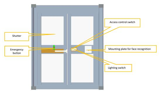
Figure 4-2-3 Internal view 01 of the front door of the container
