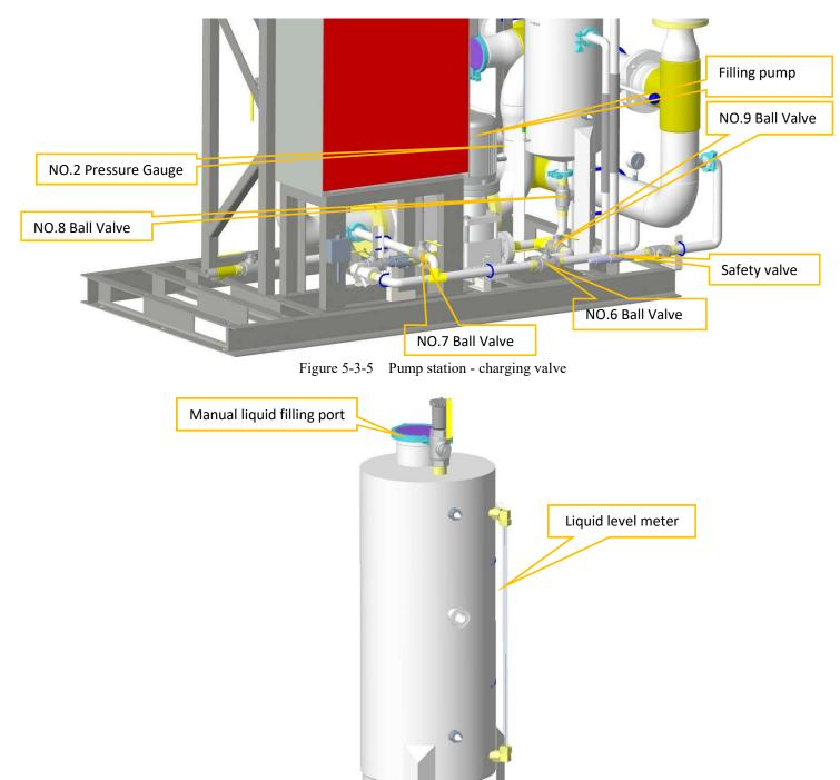
Figure 5-3-6 Pump station - liquid level meter
