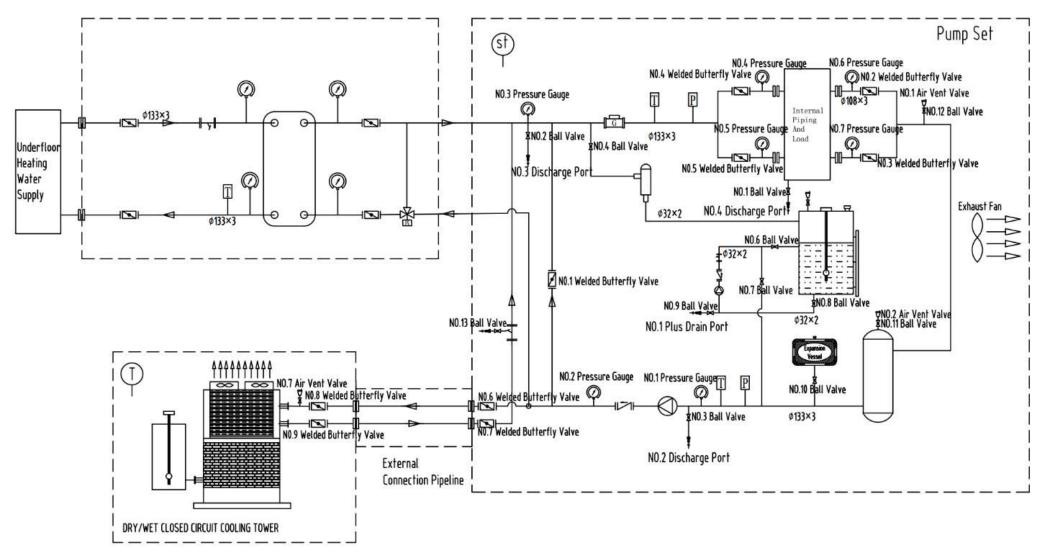
Figure 2-1 Schematic diagram of ANTSPACE liquid cooling system
