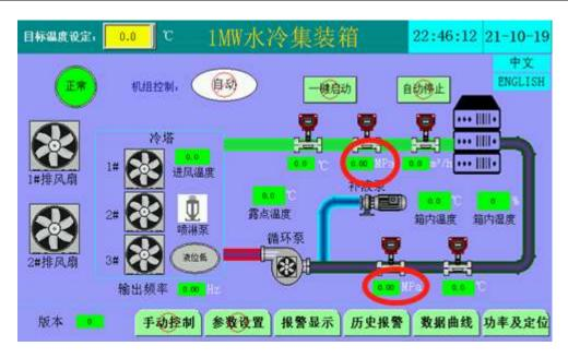
Figure 5-3-7 pressure sensor reading on main interface
