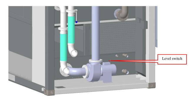
Figure 5-4-4 Installation diagram of liquid level sensor
