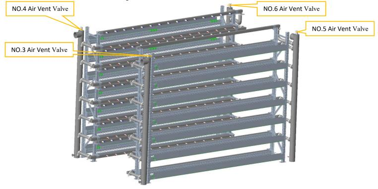
Figure 5-3-2 Manifold-Air Vent Valve
