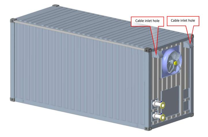
Figure 5-4-1 Cable inlet hole
