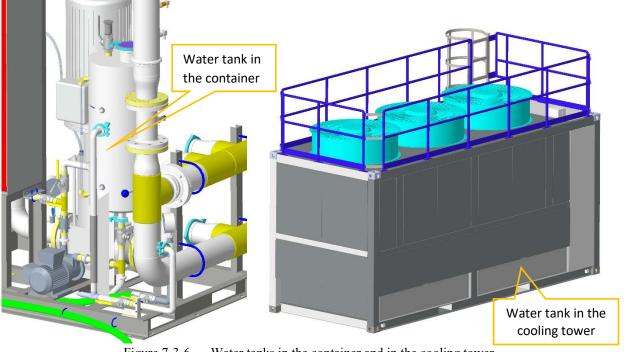
Figure 7-3-6 Water tanks in the container and in the cooling tower
