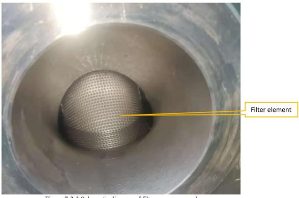
Figure 7-3-3 Schematic diagram of filter cap unscrewed
