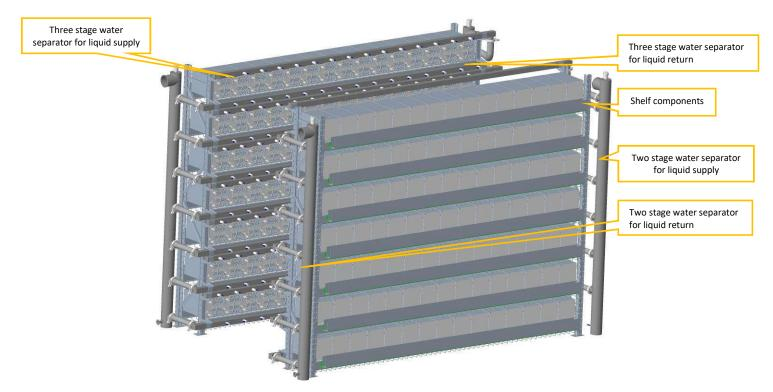
Figure 4-2-2 Internal view 01 of the water separator assembly
