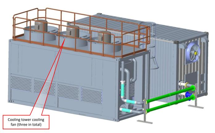
Figure 5-4-3 Location of cooling tower cooling fan
