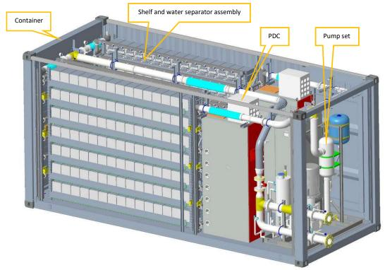
Figure 4-2-1 Internal view 01 of the container
