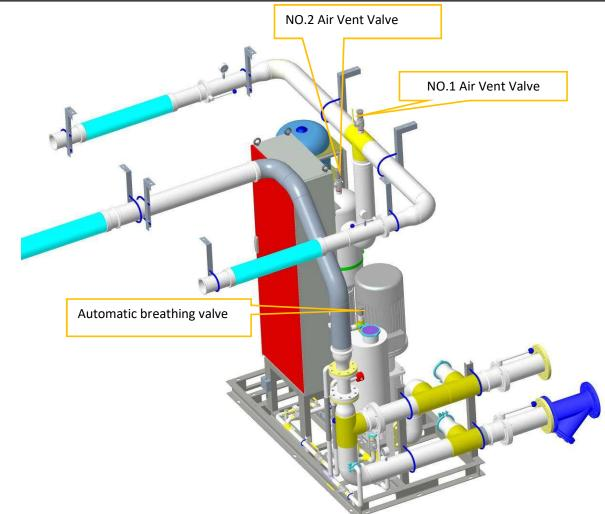
Figure 5-3-1 Internal container - automatic exhaust valve
