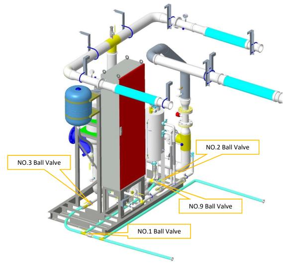
Figure 8-3-5 Filling/discharging valve for the pump station inside the container b) Connect the drain hose to No. 2 ball valve and No. 3 ball valve, tighten with a hose clamp; Lead the hose out of the unit and open No. 1-3 ball valve and No. 9 ball valve to drain the system.
